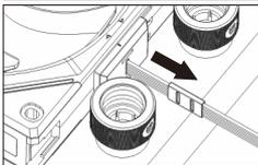
The top cover is removable if it is affected by the radiator inlet and outlet, and route the cable vertically.
